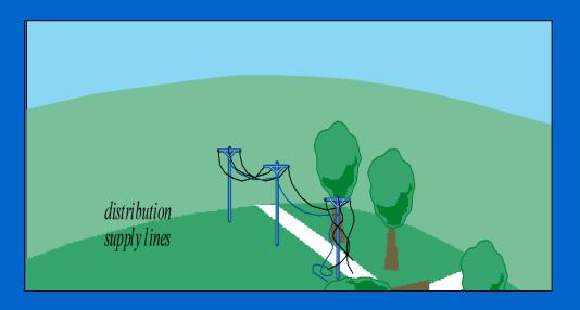
• Main distribution supply lines are checked next if the problem cannot be isolated at the substation. These supply lines carry electricity away from the substation to a group of consumers, such as a town or housing development. When power is restored at this stage, all consumers served by this supply line could see the lights come on, as long as there is no problem farther down the line.
