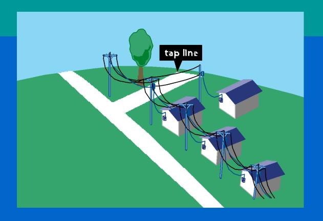
• The final supply lines, called tap lines, carry power to the utility poles or underground transformers outside houses or other buildings. Line crews fix the remaining outages based on restoring service to the greatest number of consumers.
