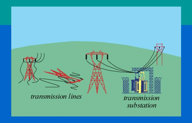
• Transmission towers and lines supply power to one or more transmission substations. These lines seldom fall, but they can be damaged by a hurricane or tornado. Tens of thousands of people could be served by one high-voltage transmission line, so if there is damage here it gets attention first.
