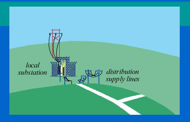
• A co-op may have several local distribution substations, each serving thousands of consumers. When a major outage occurs, the local distribution substations are checked first. A problem here could be caused by failure in the transmission system supplying the substation. If the problem can be corrected at the substation level, power may be restored to a large number of people.
